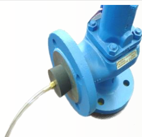
Valves seat Leakage I/T Legaline Bubble Test (10)
