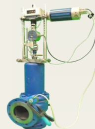
On Line Safety Relief Valves I/T »Legatest» (07,08)
