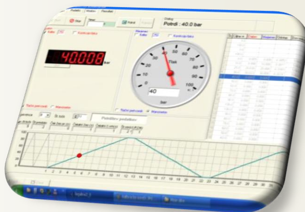
Manotest software: Calibration of pressure gauge. Part of Calibration Report (Resultants)
