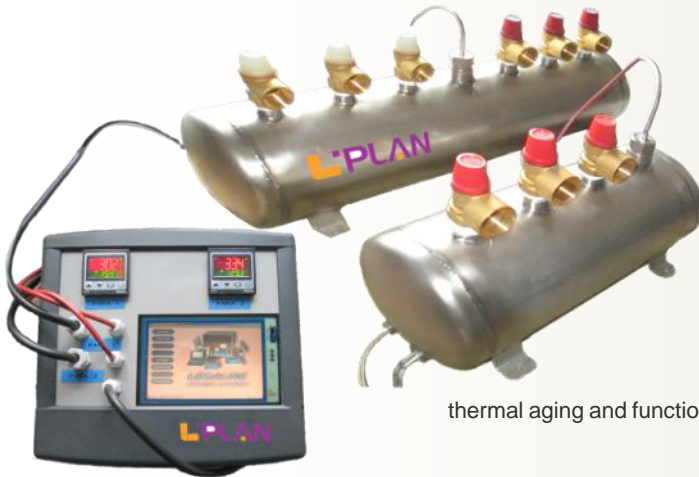
valve cyclic and tightness test,
