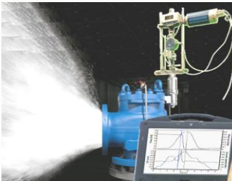
Pilot Assisted Safety Valves T. Legatest (08)
