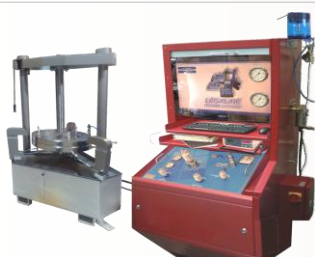
Safety / Industrial Valves I/T Stabile Test units (11, 12)
